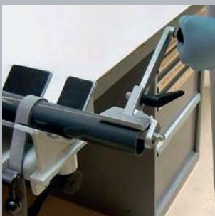
Cut chamfer and deburr the pipe
