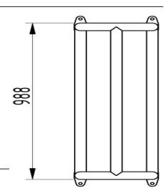
Functional and robust in design, AUTOPA's range of column protectors are designed to protect corners, columns, and other vulnerable pillars from vehicle damage in a busy industrial environment. Our Column Protectors are manufactured from mild steel and galvanised to ensure their longevity. Suitable for both internal and external use.
