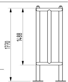
Functional and robust in design, AUTOPA's range of column protectors are designed to protect corners, columns, and other vulnerable pillars from vehicle damage in a busy industrial environment. Our Column Protectors are manufactured from mild steel and galvanised to ensure their longevity. Suitable for both internal and external use.
