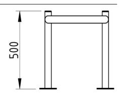
Functional and robust in design, AUTOPA's range of column protectors are designed to protect corners, columns, and other vulnerable pillars from vehicle damage in a busy industrial environment. Our Column Protectors are manufactured from mild steel and galvanised to ensure their longevity. Suitable for both internal and external use.
