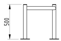
Functional and robust in design, AUTOPA's range of column protectors are designed to protect corners, columns, and other vulnerable pillars from vehicle damage in a busy industrial environment. Our Column Protectors are manufactured from mild steel and galvanised to ensure their longevity. Suitable for both internal and external use.
