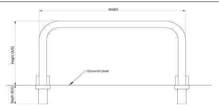
Perimeter Barriers are designed to help secure site perimeters and provide a permanent obstacle to vehicle access, to mark boundaries, define trolley parks and protect vulnerable door entrances and exits.
