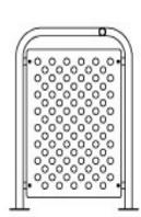
AUTOPA Door Guards are designed to protect walls from being damaged by swinging doors. An integrated rubber stopper acts as a shock absorber, preventing the door from hitting the steel frame. Ideal for commercial and industrial sites, they are suitable for internal and external use and can be installed either individually or in pairs.
