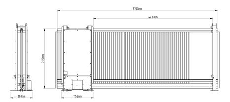
This is the drawing for the AUTOPA Automatic sliding gate. It shows the dimensions of the system but does not take into account any additional dimensions that will need to be considered such as that of the induction loop that is installed into the ground next to the system. Please take into these extra dimensions when thinking of where this system will be installed, as suitable requirements will need to be met for it to be properly installed and have suitable operation.
