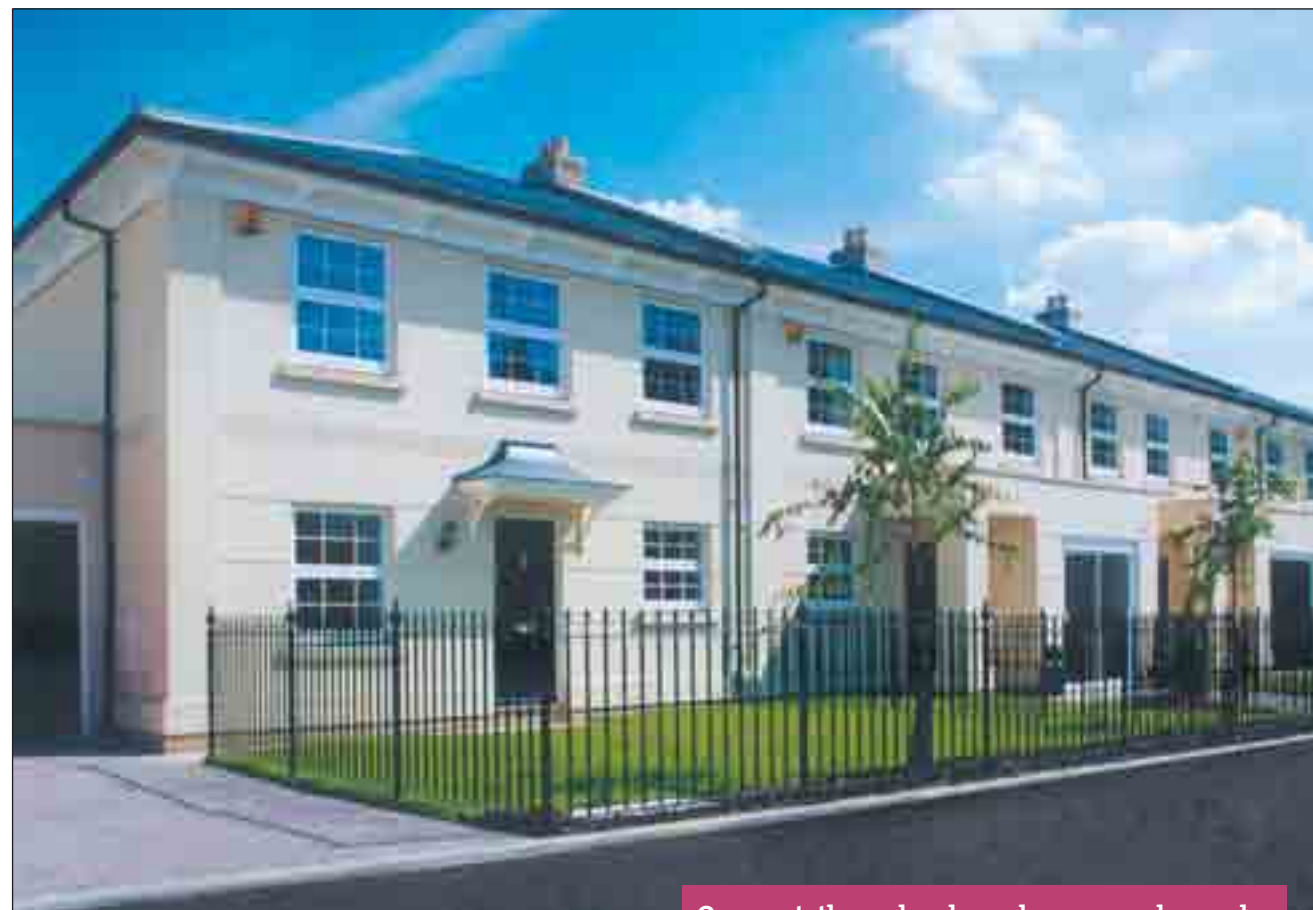
One-coat, through-coloured monocouche render
