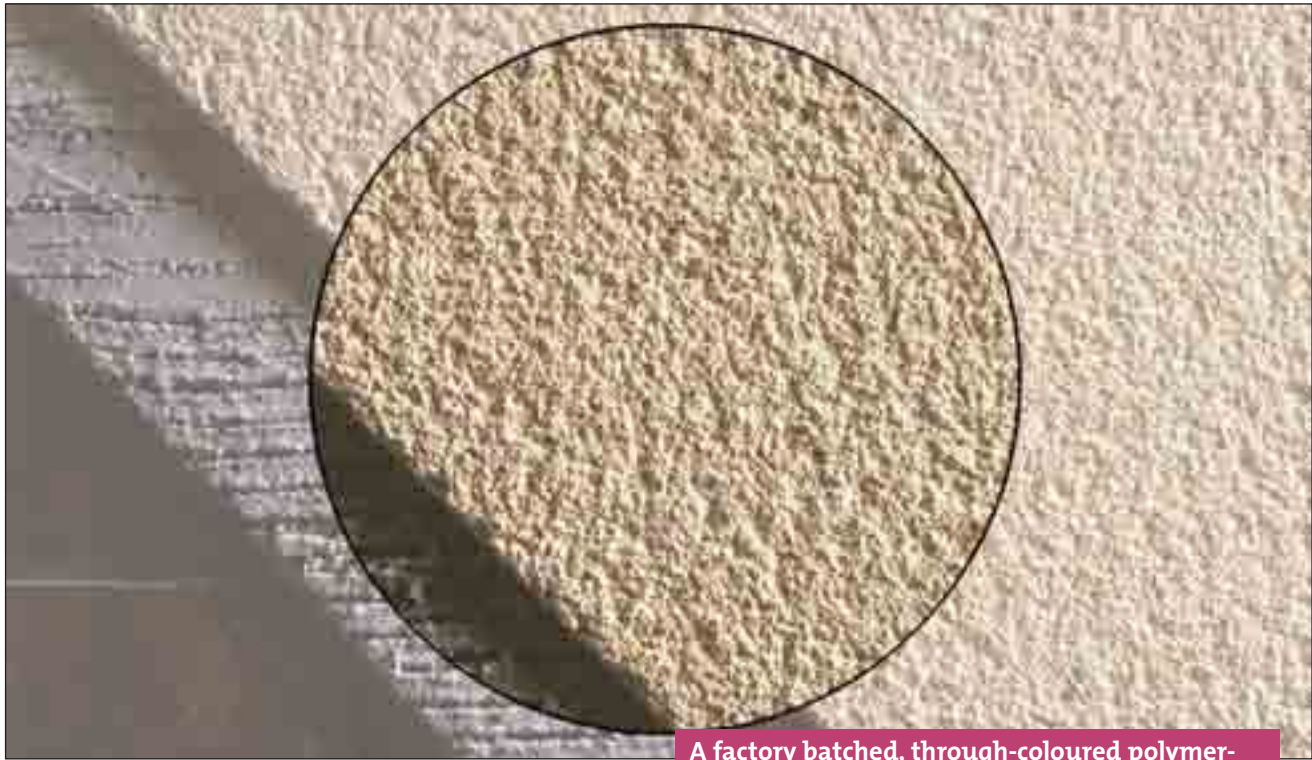
A factory batched, through-coloured polymer-modified mortar for use as a render top coat
