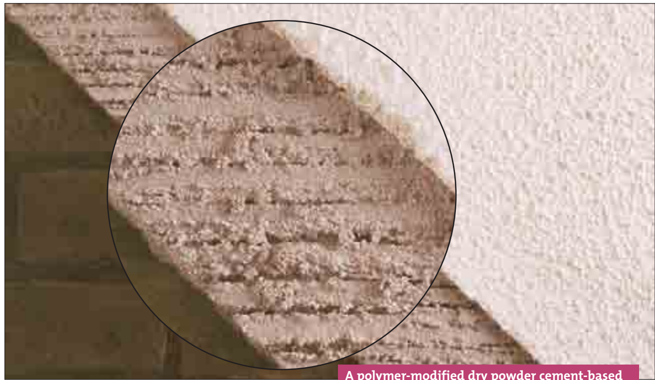
A polymer-modified dry powder cement-based mortar for use as a render undercoat
