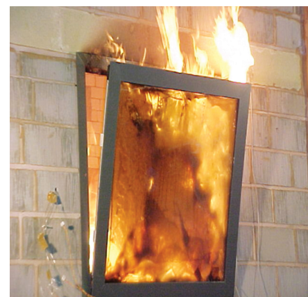
EN 12101 Part 02 Annex G testing prescribed for automatic smoke vents
