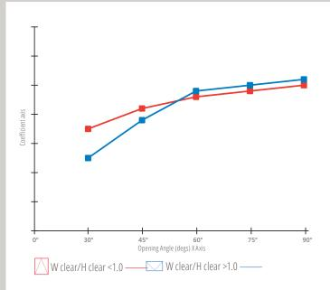
The different results are relative to the aspect ratio of the vent width / height.
