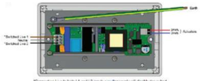
\*Connecting Live to both L1 and L2 inputs simultaneously will disable the output
