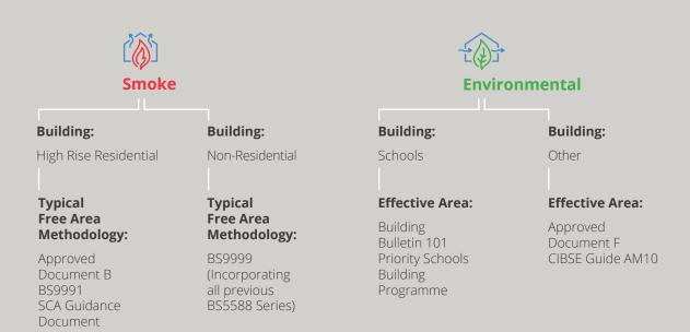
There are generally three methods to measure free area through a vent which are applied relative to the building type and the application (smoke or environmental ventilation).
