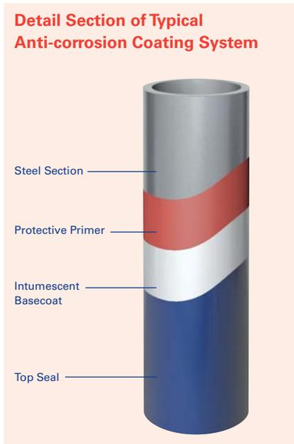
Combine Nullifire Primers and Top Seals with Nullifire Intumescent Basecoats to provide a complete system for fire protection and then decoration of structural steel. All Nullifire products are tested for compatibility to minimise the risk of problems occurring on site.
