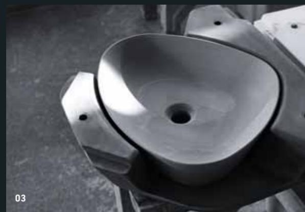
**01** Plaster moulds give bathroom ceramics their shape. At the same time, the plaster coating removes water from the slip and allows the ceramic bodies to develop.
