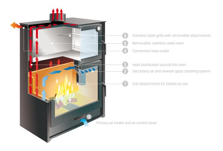
Aranda wood-fired oven is fully built in cast iron, with a stainless steel oven and oven light.
