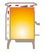
Double convective body: the double cast iron body and heat exchanger maximize the heating surface of the stove and the convection heat ensures a gentle warmth while keeping a powerful heat output. (Manchester and Bennington models).
