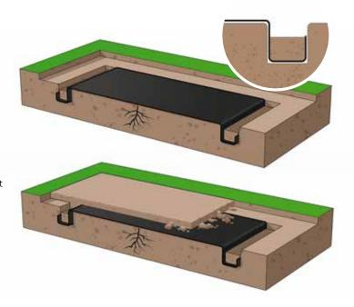
Proper use of Plantex\* Platinium nonwoven fabric requires attention to the recommended installation guidelines. The product may be installed horizontally either on flat land - or on slightly sloped embankments, in which case additional considerations may be required. The joining of separate lengths should be achieved either by the DuPont recommended thermal-welding technique or by the use of Plantex\* Performance Tape.
